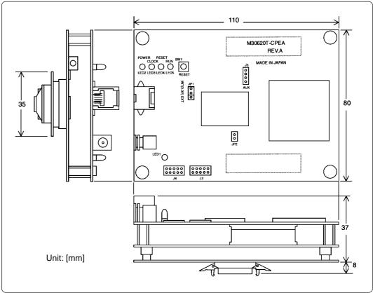
Figure 4.3 External dimensions of emulator
